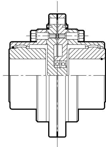
**Shear Pin Gear Coupling**
