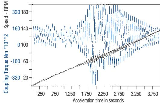
Table C shows a typical motor/fan system connected rigidly (or through a gear or membrane coupling) when damaging torques would have been experienced in the motor shaft.
