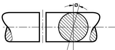
Torsional flexibility is a design feature necessary to permit shock and impulsive loadings to be suitably dampened. It is achieved by the provision of a flexible medium such as rubber, springs, etc., between the two halves of the coupling.
