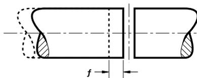
End float is the ability to accommodate a relative axial displacement of the connected shafts; achieved by sliding members or flexing of resilient components.
