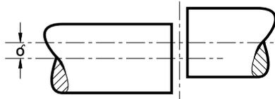
Axial misalignment is present when the axes of the driving and driven shafts are parallel but laterally displaced.
