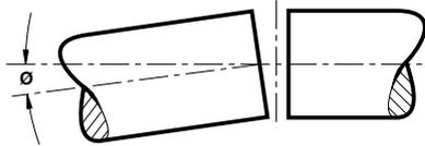
Angular misalignment is present when the shaft axes are inclined one to the other. Its magnitude can be measured at the coupling faces.
