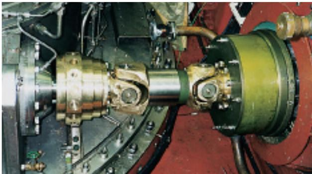
Renold Hi-Tec Couplings has a unique capability to design and manufacture special couplings.
