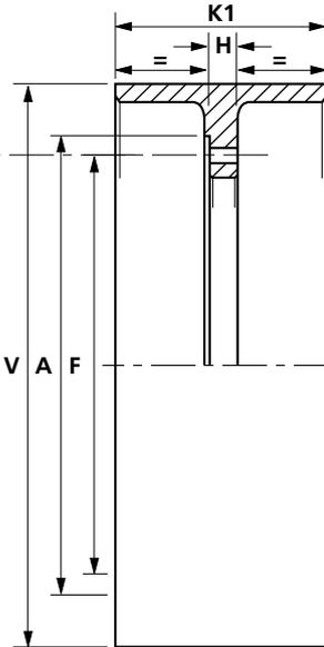
Brakedrums may be used in conjunction with the whole range of PM couplings and may be bolted on either the driving flange or flexible half side of the coupling, the recess -  $\varnothing A$  - locating on the outside diameter of the coupling.
