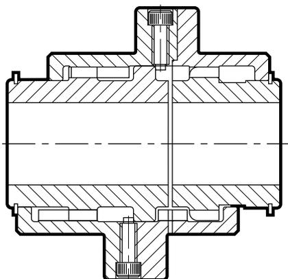
**Disengaging Type Gear Coupling - Standard Series**
