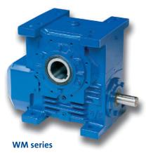
Worm gear units are available with imperial 4" - 9" centres and metric 100mm - 200mm centres with power capacities up to 115kW. Available with ratios of 5:1 to 70:1 as a single reduction unit and 75:1 to 4900:1 as a double reduction.
