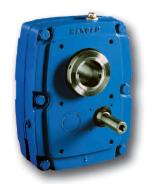
Shaft mount helical gear units available with a hollow output bore, in 12 sizes with 5 ratio options per size. Power capacities up to 235kW.
