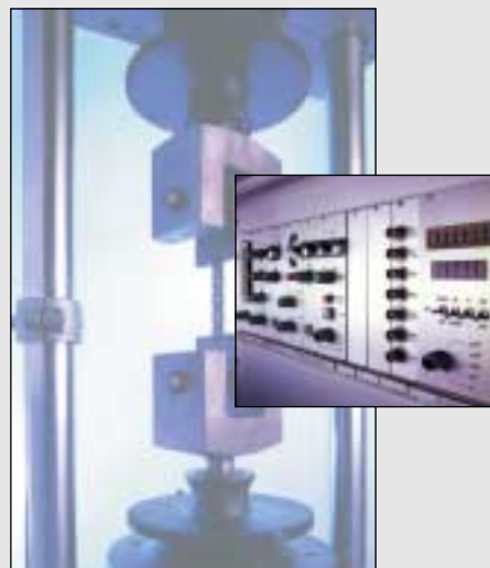
For the testing of fatigue strength, we use, among others, this – designed according to the latest technological knowledge – high frequency fatigue testing machine.
